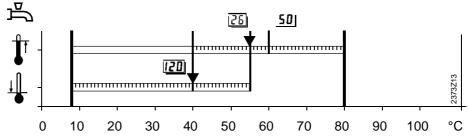
Setting "Nominal setpoint of the d.h.w. temperature"Setting "Reduced setpoint of the d.h.w. temperature"
